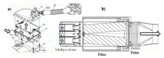
Fig. 1. Schematic view of a Panel Filter- a) Direct Flow filter- b)
