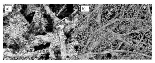
Fig. 5. Dust particle distribution on cellulose filter media -a) and on nanofiber filter media -b)
