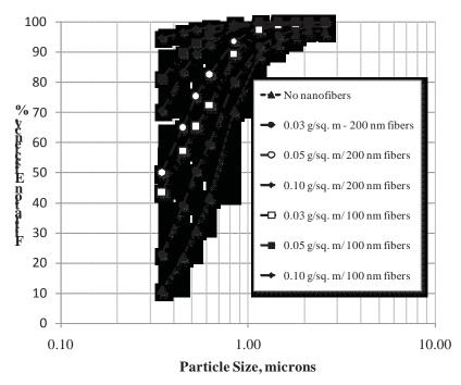
Fig. 6. Fractional efficiency vs. particle size (microns) for various basis weight of nanofibers applied to a cellulose substrate
